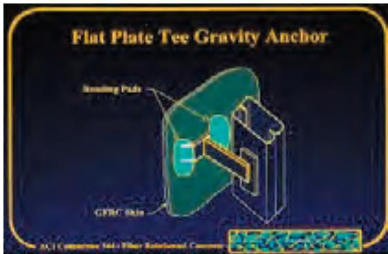
Figure 20 - Flat plate tee gravity anchor
