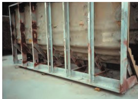
Figure 16 - Heavier frames now galvanized
