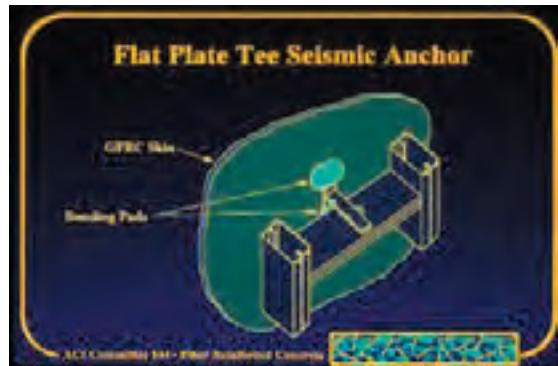
Figure 21 - Flat plate tee seismic anchor
