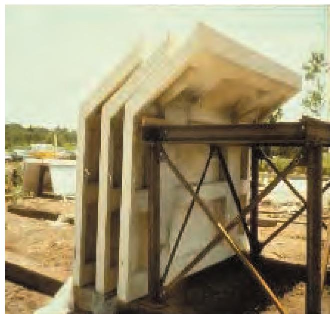
Figure 3 - Early rib design (foam core)
