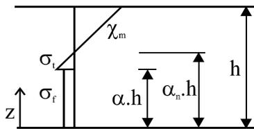
**Figure 11:** Stress distribution in a cracked section subject to bending
