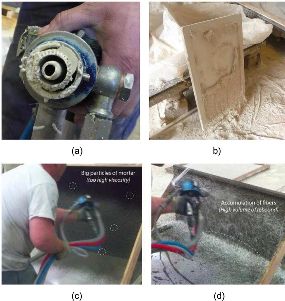
**Figure 4:** Examples of rheological problems to due to inadequate viscosity (too high)
