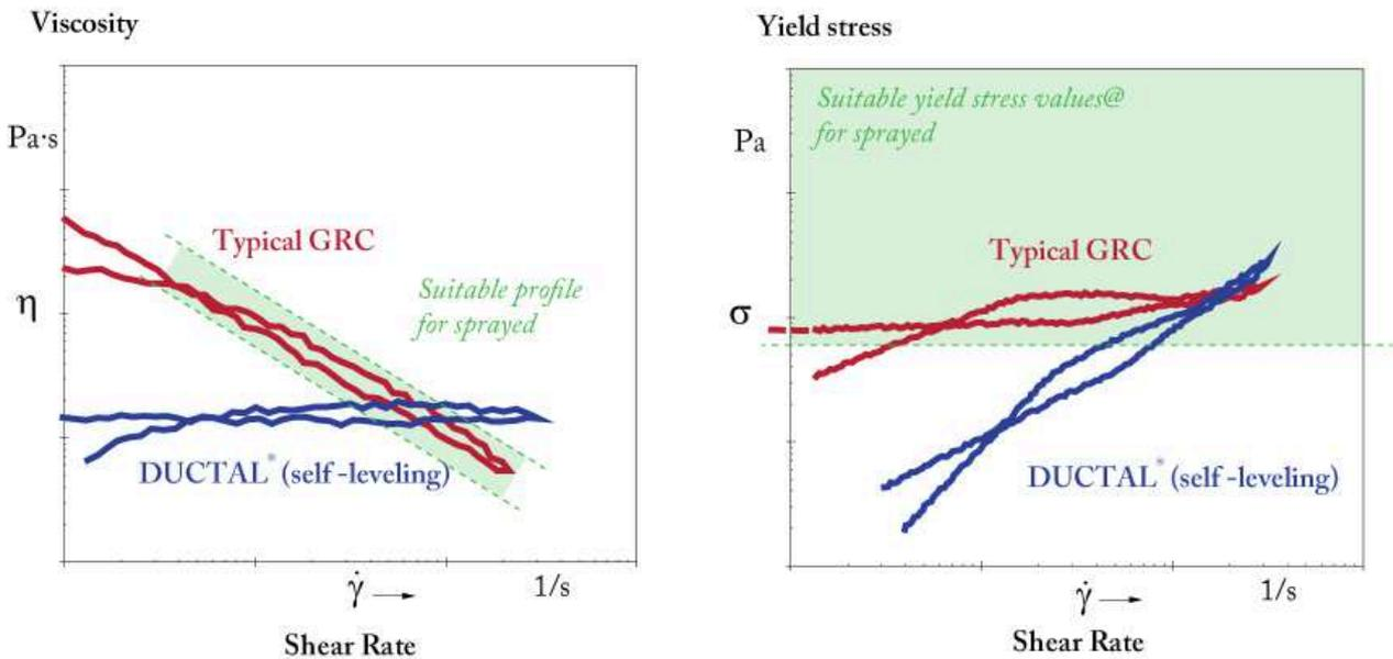
**Figure 5:** Rheological profile comparison between a self-leveling Ductal® and typical GRC
