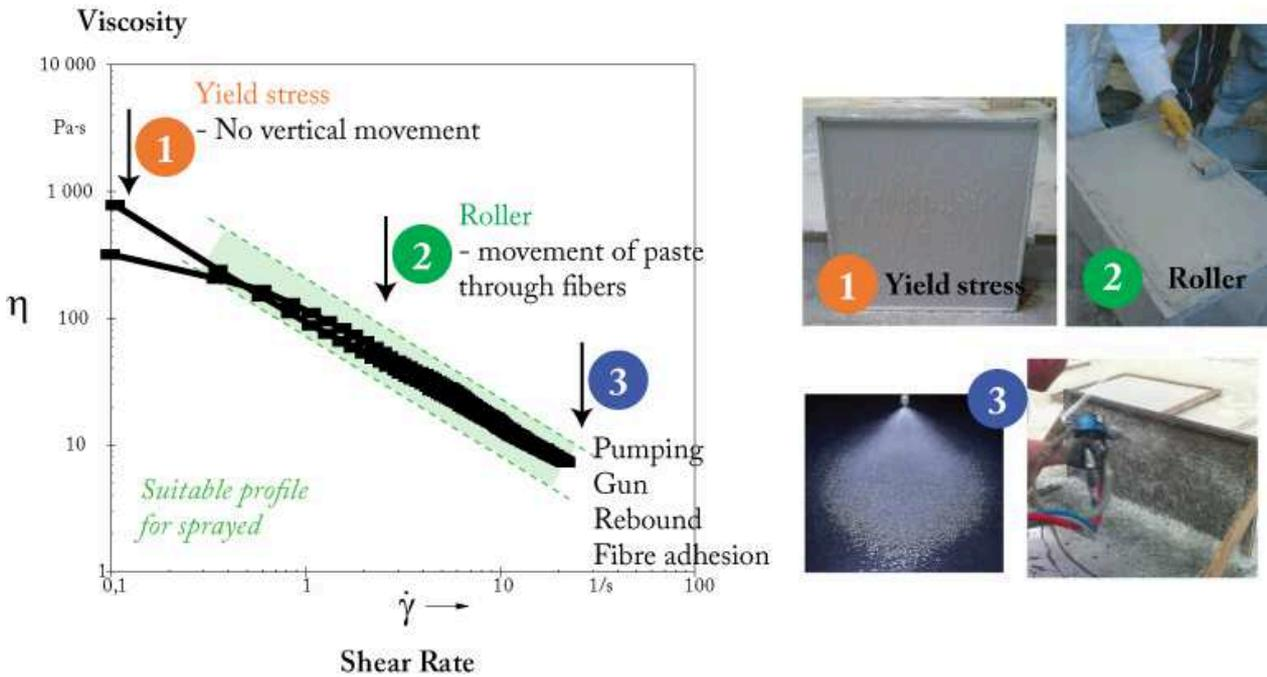
**Figure 3:** Schematic description of expected rheological profile for the GRC process
