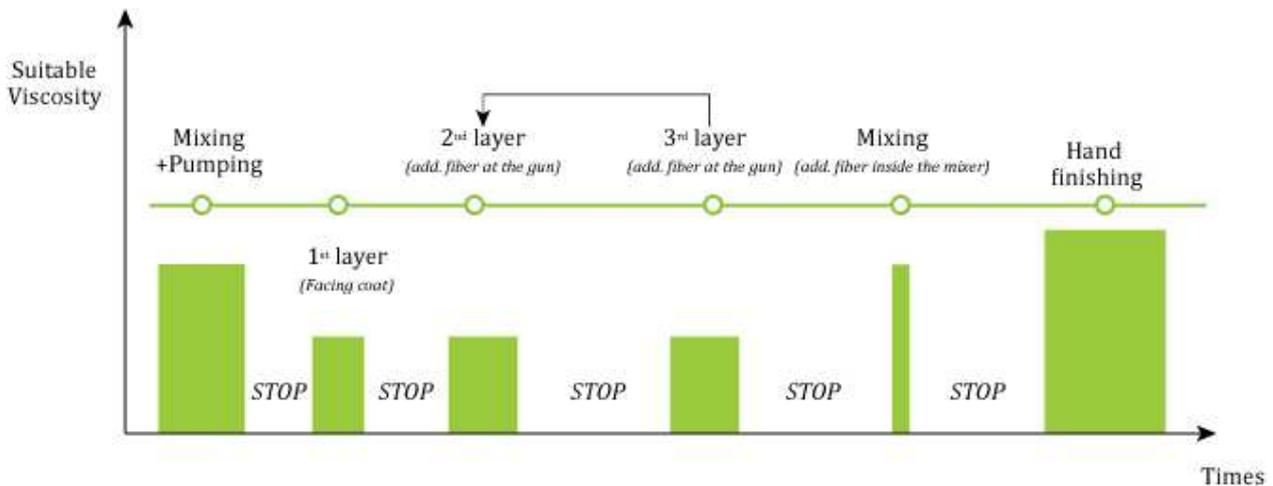
**Figure 2:** Schematic representation of the shotcreting process expectation in terms of suitable mortar viscosity over the times.
