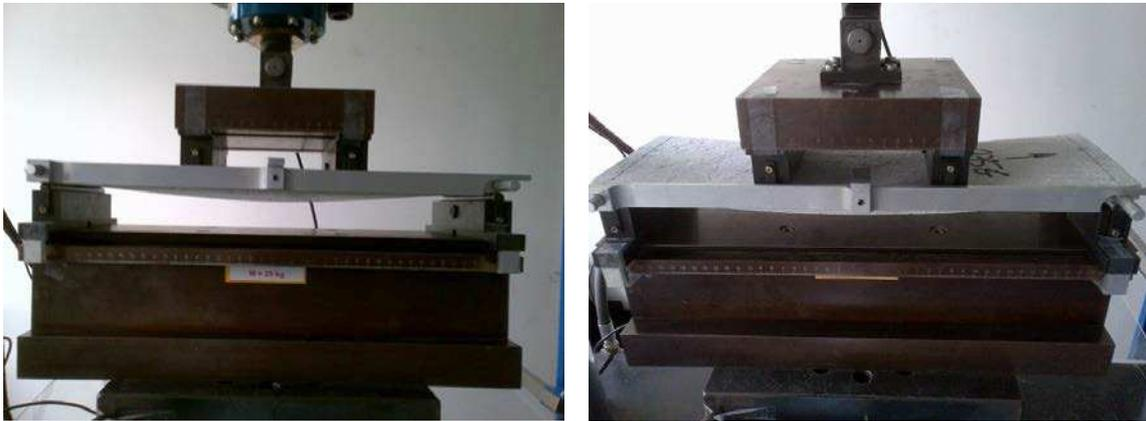
**Figure 8:** Four bending test. Example of deflection observed with sprayed Ductal<sup>®</sup> mixes at 28d
