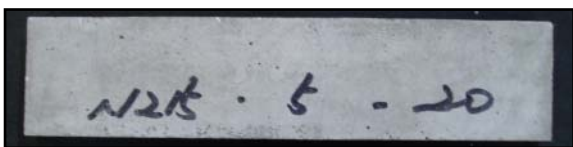
Photograph 4. Freezing and thawing test specimen (No.13, 300c)
