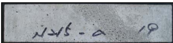
Photograph 3. Freezing and thawing test specimen (No.10, 100c)
