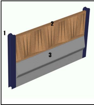
Figure 5: Design of sound protection wall RW03
