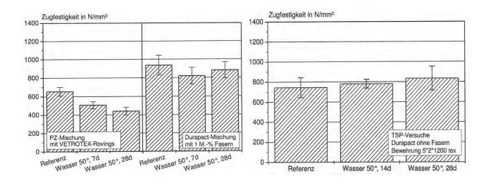
The diagram shows the results of a accelerated test, specimen were deposited in water  $50^{\circ}\,\text{C}.$
