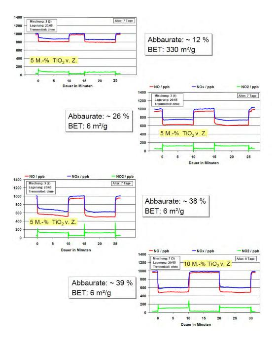
Generally a white matrix shows more degradation of air-purifying and the w/c - ratio has influence too. Is that ratio higher the degradation rate is less. Other factors of influence are the time of demoulding and the curing. For example there was no degradation rate measured when the specimen were stored 7 days in water.
