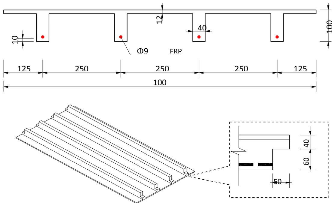
**Figure 9** Error! No text of specified style in document. Dimension and isometric view of the designed formwork
