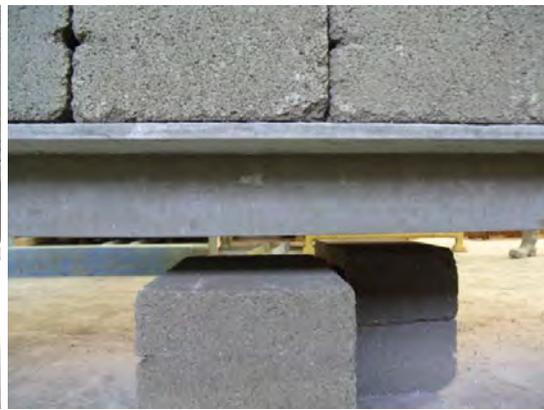
Figure 12 Evenly distributed fine cracks
