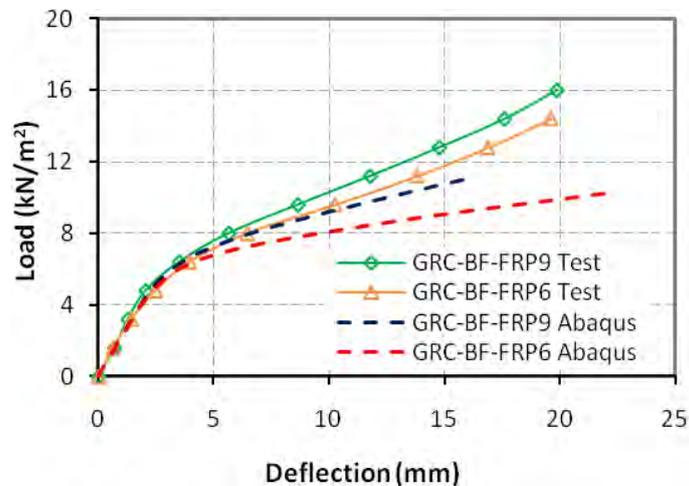
Figure 18 Predicted and measured load-deflection response of FRP reinforced formwork
