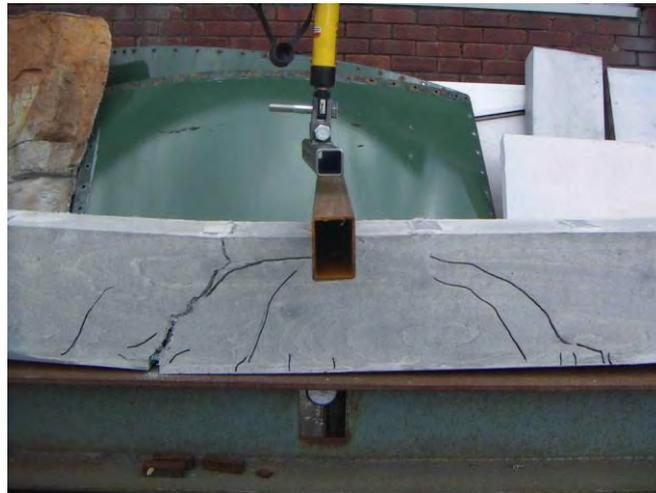
Figure 6 Test setup and failure pattern
