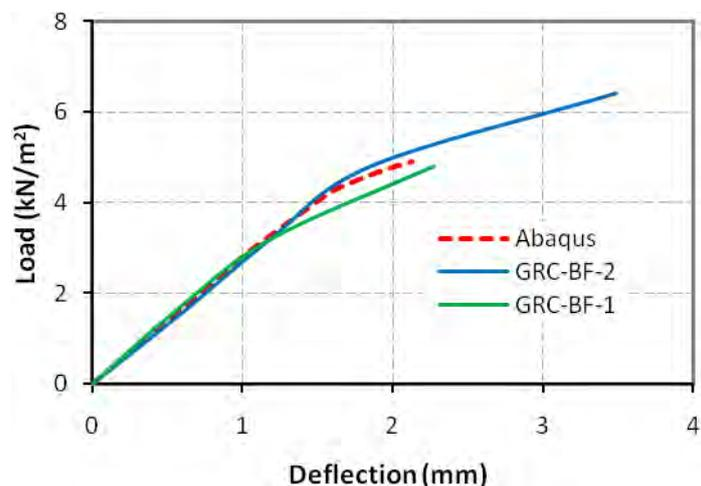
Figure 17 Predicted and measured load-deflection response of unreinforced formwork
