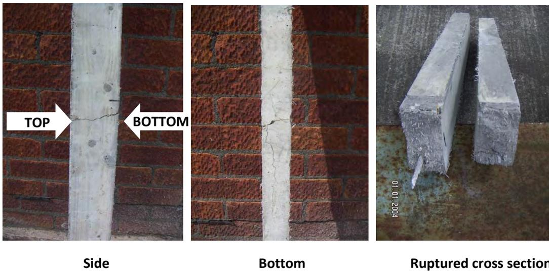
Figure 3 Failure pattern
