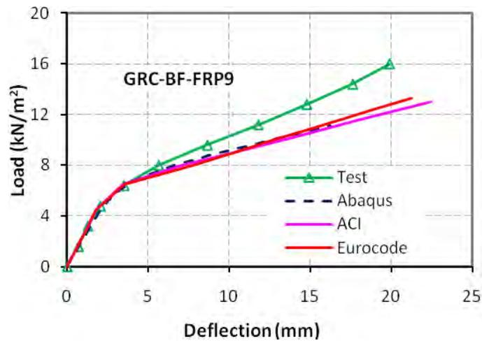
Figure 20 Comparison of load-deflection relationship among test, FE analysis and code prediction for formwork GRC-BF-FRP9
