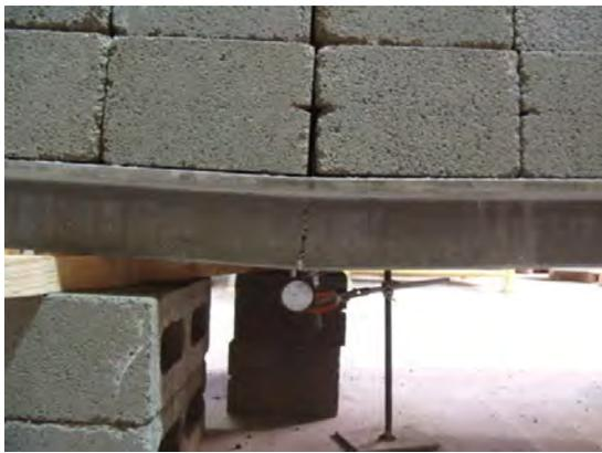
Figure 11 Failure of GRC unit
