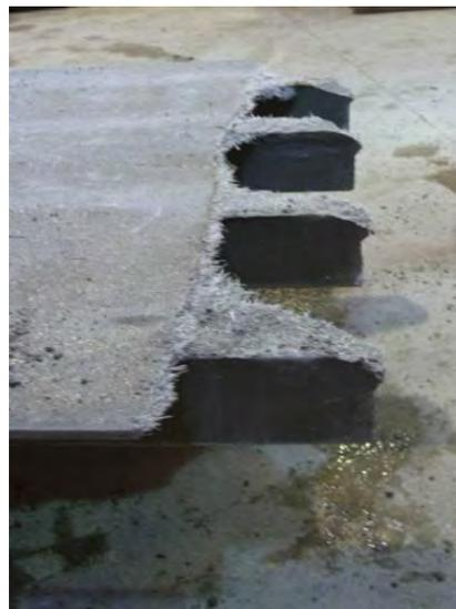
Figure 14 Shear failure
