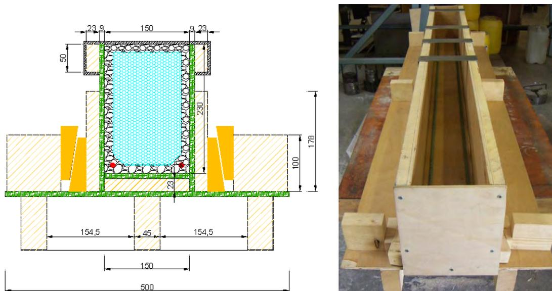
Figure 5 Mould dimension and finished mould
