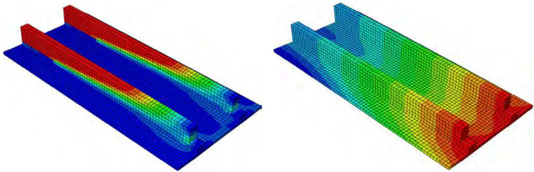
Figure 16 Stress and vertical deflection of GRC-BF-FRP9
