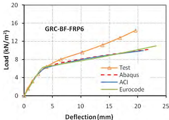
Figure 19 Comparison of load-deflection relationship among test, FE analysis and code prediction for formwork GRC-BF-FRP6
