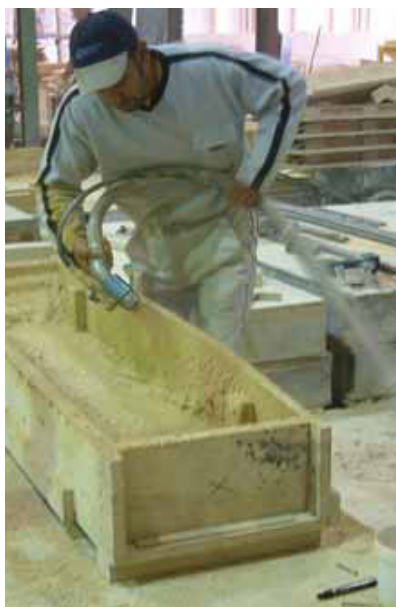
Figure 1: With sprayed premix, the fibre is added to the matrix during the mixing process and the mixed fibre and matrix are pumped to a spray gun and sprayed onto the mould.
